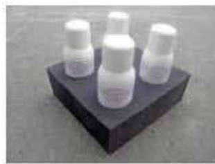
RCT-1031 vials, set of 4, for testing fresh concrete
